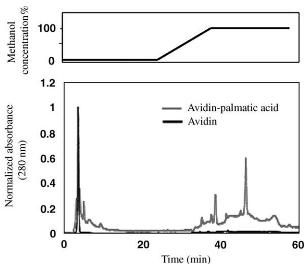
Fig. 2. Palmitoylated avidin verified by reverse-phase HPLC (C18 column) with a methanol gradient in the mobile phase. Palmitoylated avidin was eluted of the column with a linear gradient of methanol in 1 × PBS.
