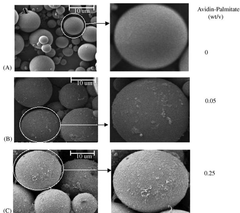
Fig. 4. Surface microtopography correlates with increasing concentrations of avidin–palmitate in the emulsion. Representative examples of three batches with (A) 0, (B) 0.05, and (C) 0.25 w/v avidin–palmitate in a 5% PVA emulsion.
