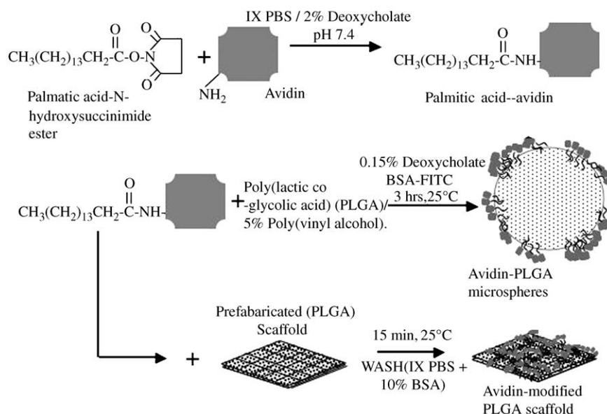
Fig. 1. Overall scheme depicting the modification of PLGA particles and scaffolds with palmitoylated avidin. (A) Conjugation of palmitic acid to avidin and (B) incorporation of avidin-palmitate on the surface of PLGA particles using the double emulsion-solvent evaporation method. Surface modification of scaffolds was more direct with avidin-palmitate added directly to the PLGA matrix followed by a washing step in blocking buffer.
