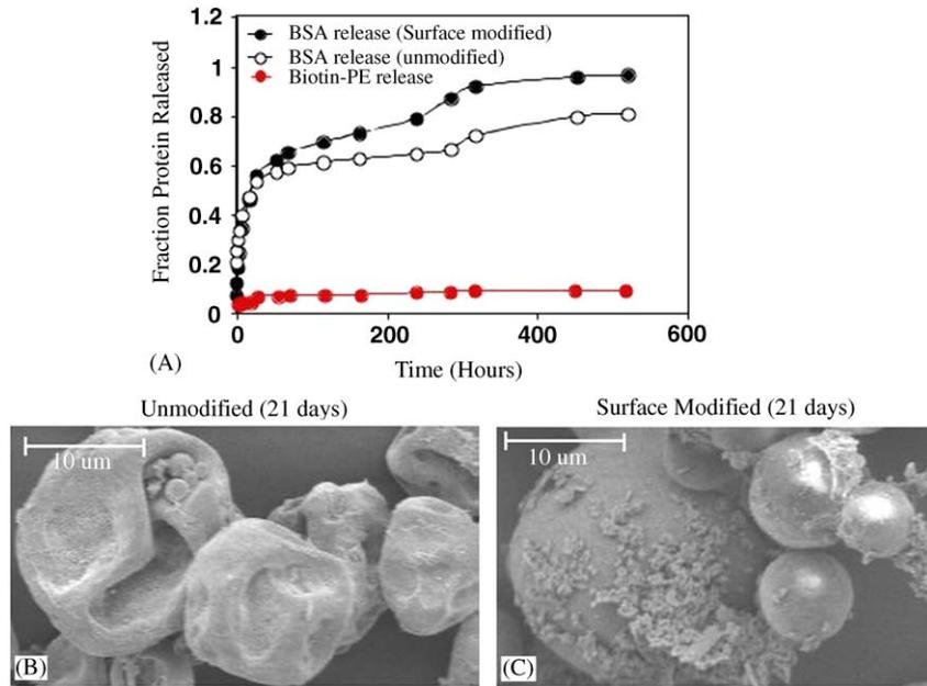
Fig. 8. Controlled release of BSA and surface biotin-PE from modified microspheres and comparison to release of BSA from plain microspheres. (A) Controlled release experiment in 1 × PBS and 37 °C for 25 days. (B, C) SEM images of degraded plain and modified microspheres (21 days).
