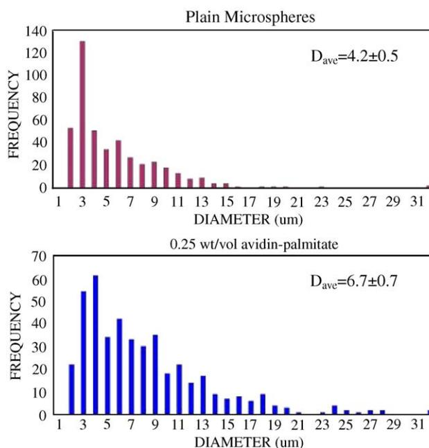
Fig. 3. Particle size distribution analysis of (A) plain and (B) modified PLGA particles. Particle size distributions were based on SEM images and performed with NIH SCION<sup>®</sup> image analysis software.
