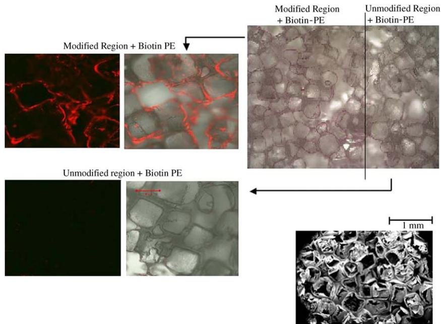
Fig. 9. Regional surface modification of PLGA scaffolds with avidin–palmitate followed by biotin-PE staining. Fluorescence and phase contrast comparison of modified and unmodified regions on the same scaffold.
