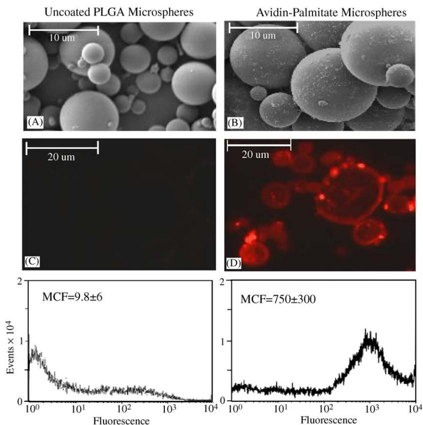
Fig. 5. Comparison of surface staining with biotin-PE for both plain (A, C, E) and modified particles (B, D, F). Fluorescence imaging of particles (C, D) and flow cytometry (ungated) of modified and plain particles (E, F). MCF is the mean channel fluorescence of FL2 (red channel).
