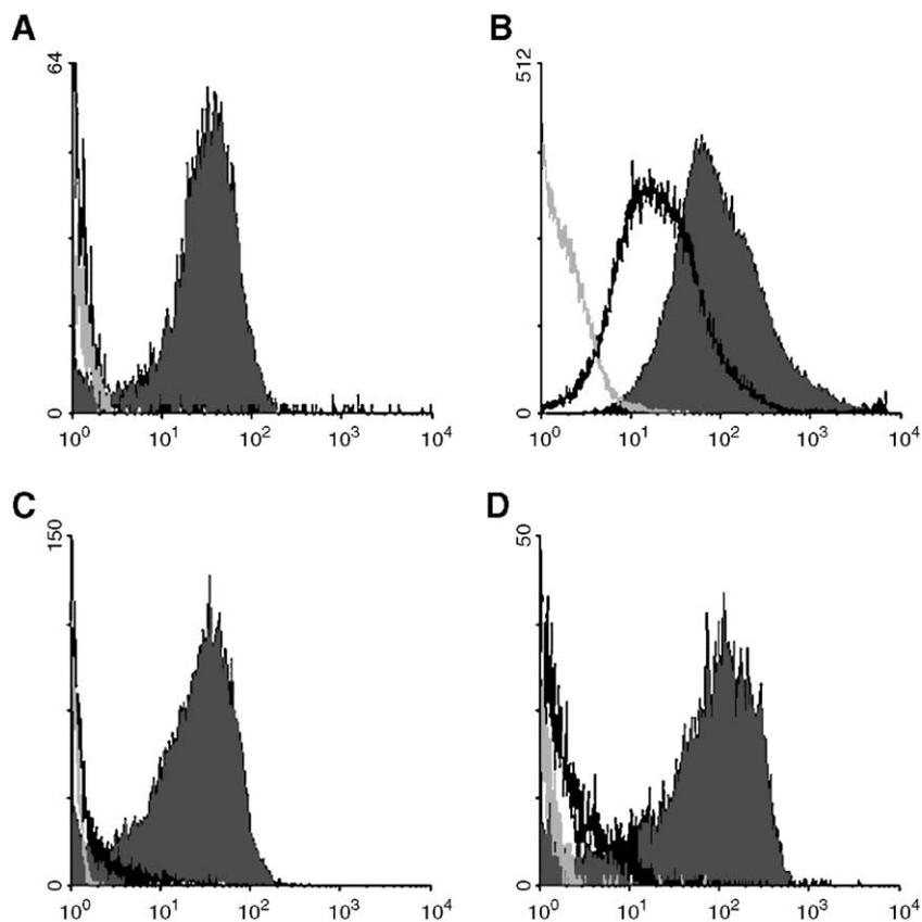
Fig. 2. Detection by flow cytometry of (A) BSA, (B) streptavidin, (C) goat-anti-mouse IgG antibody, and (D) UEA 1 conjugated to microspheres. Data are histograms of PE fluorescence. Gray line: microspheres before incubation with fluorescent label. Black line: controls for nonspecific binding of fluorescent label to microspheres. Solid fill: microspheres incubated with fluorescent labels specific for conjugated protein.
