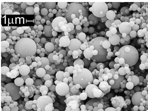
Fig. 1. Scanning electron micrograph of PLGA/PEMA microspheres with encapsulated FITC-BSA.
