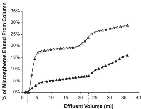
Fig. 4. Retention of goat anti mouse IgG-conjugated microspheres on agarose columns.  $\Delta$ =agarose-biotin column.  $\blacktriangle$ =agarose-mouse IgG column. Solid arrow: addition of microspheres to column. Dotted arrow: switch in elution buffer to 6 M guanidine HCl.
