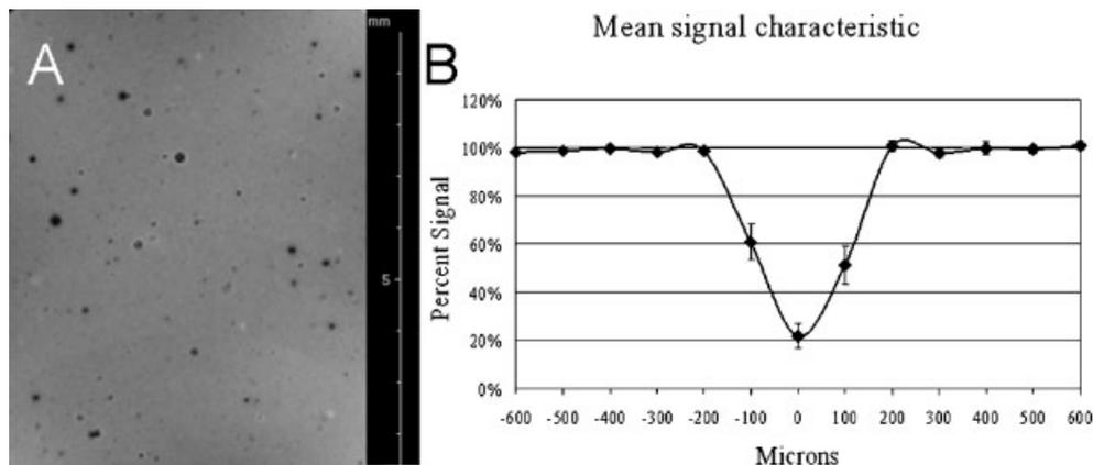
**Figure 5.** (A) MRI slice from the labeled lymphocyte phantom showing isolated, punctate, dark contrast spots. The barscale is in millimeters. (B) A mean plot profile through 12 spots, measuring the linear size and percentage contrast generated by labeled lymphocytes in the MRI experiments performed here.
